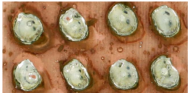
Contamination conventional solder wire
