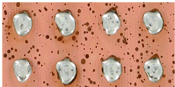
Spitting behaviour conventional solder wire
